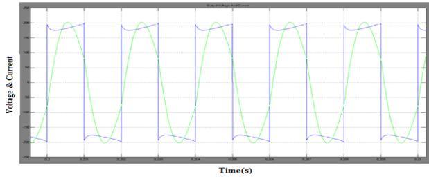
Fig.:- (B) output voltage and current of the inverter-
