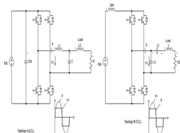
Fig. 2.1- VSI with Inductive Coupling (topology A) and CSI with capacitive coupling (topology B) of the load
