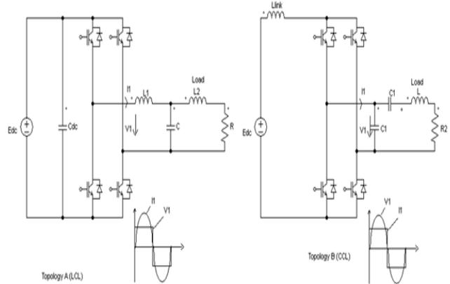
Fig. 2.1- VSI with Inductive Coupling (topology A) and CSI with capacitive coupling (topology B) of the load
