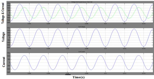
Fig.:- (D) shows the total output voltage & current across the tank coil.
