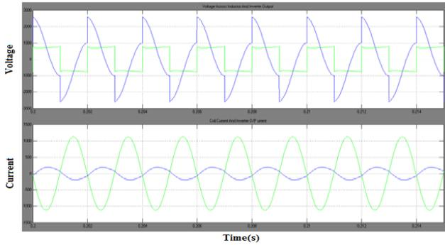
Fig.:- (C) output voltage and current across the inductor L1
