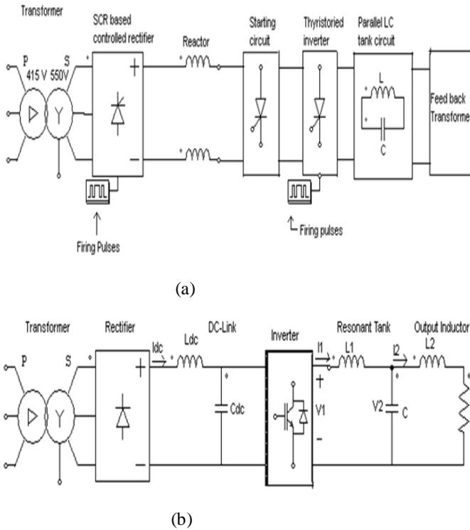
Fig. 5.1- Power schematic of (a) thyristorised based parallel resonance circuit configuration, (b) IGBT based LCL resonance inverter.
