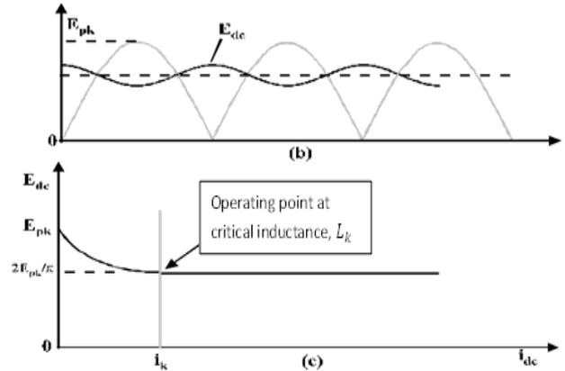
Fig. 3.1 Full wave rectifier with inductor input filter
