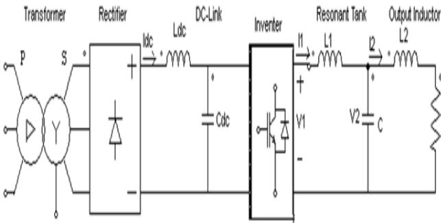
Fig.2.2- Power schematic of the IGBT based resonant inverter with LCL configuration
