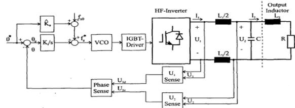
Fig. 6.1. Basic Phased Locked Loop Structure
